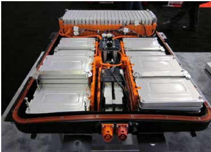
This is a photo of the Nissan Leaf's li-ion battery pack. The Leaf was introduced in 2011 as the first mass-produced EV sold in the U.S. In 2026, Nissan will begin building two new EV models at its plant in Canton, Mississippi.
